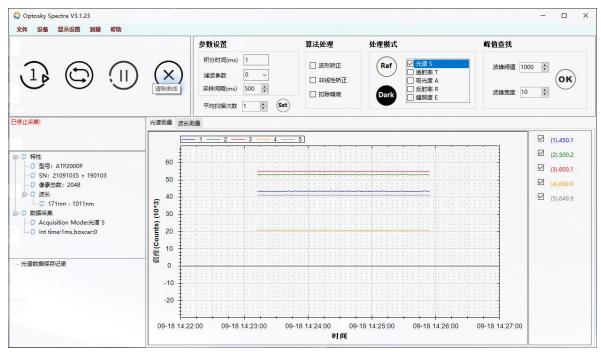
Figure 2 Output power stability of ATG1300 (change rate <0.13%)
