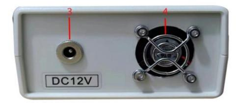
1 light source switch, 2 optical fiber interface, 3 power interface (DC12V), 4 cooling fan
